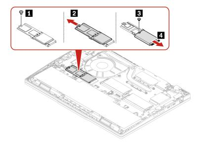
Step 2. Install the 2242 M.2 solid-state drive and its bracket in reverse order.
