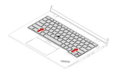
Step 3. Pivot the keyboard slightly upward I and then turn over the keyboard 2.
