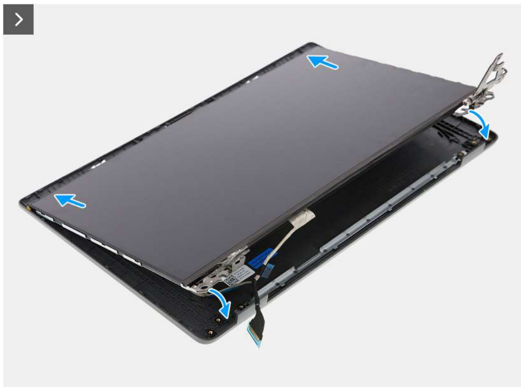
Figure 63. Installing the display panel
