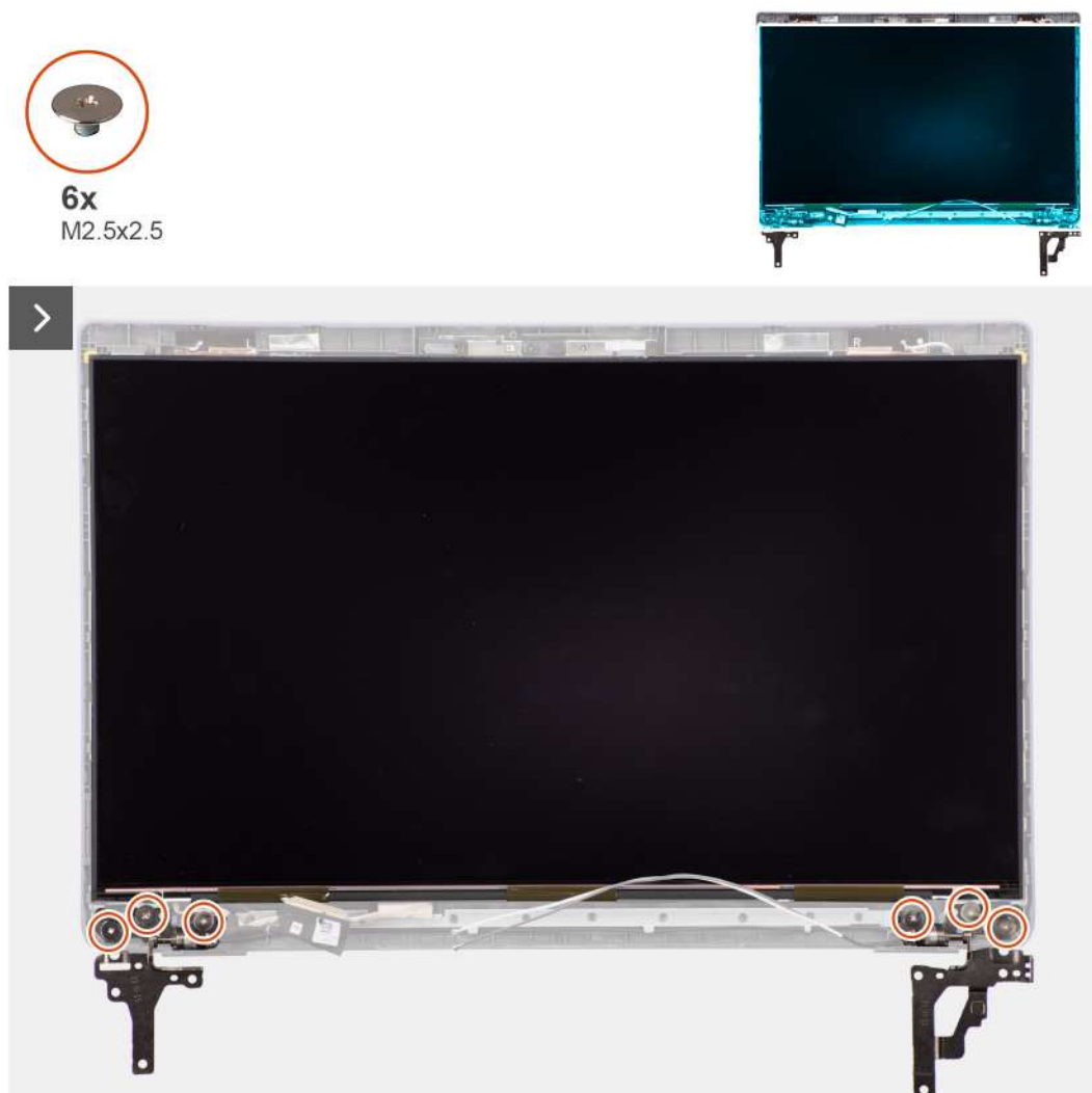
Figure 56. Removing the display panel
