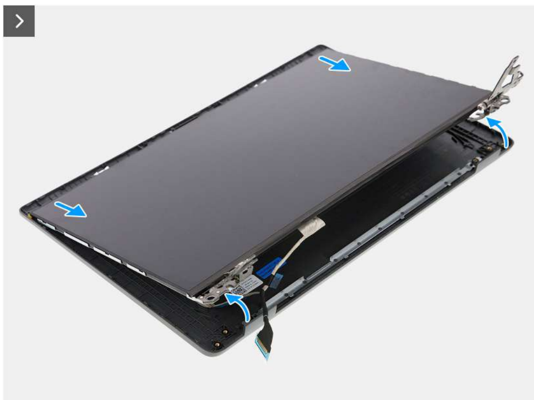
Figure 58. Removing the display panel
