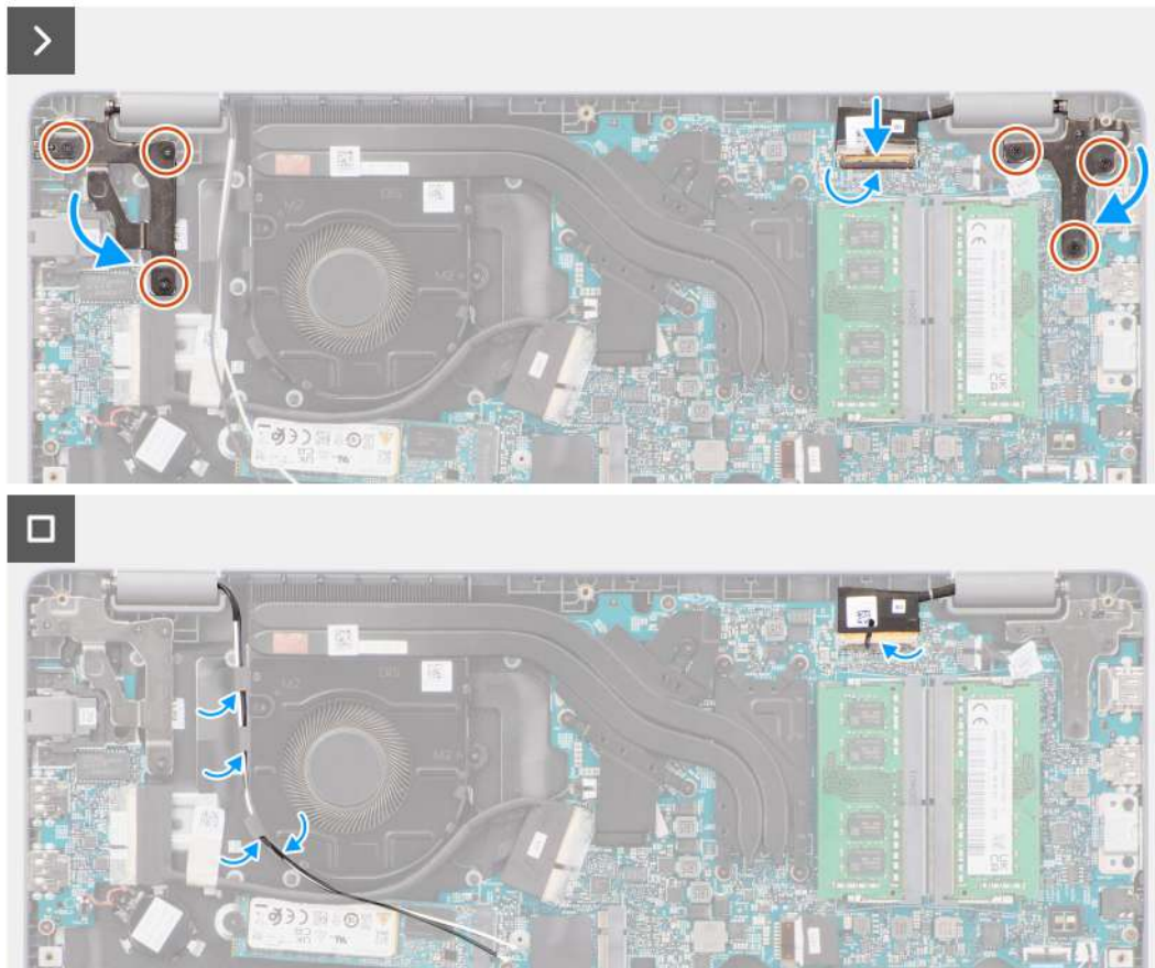
Figure 52. Installing the display assembly
