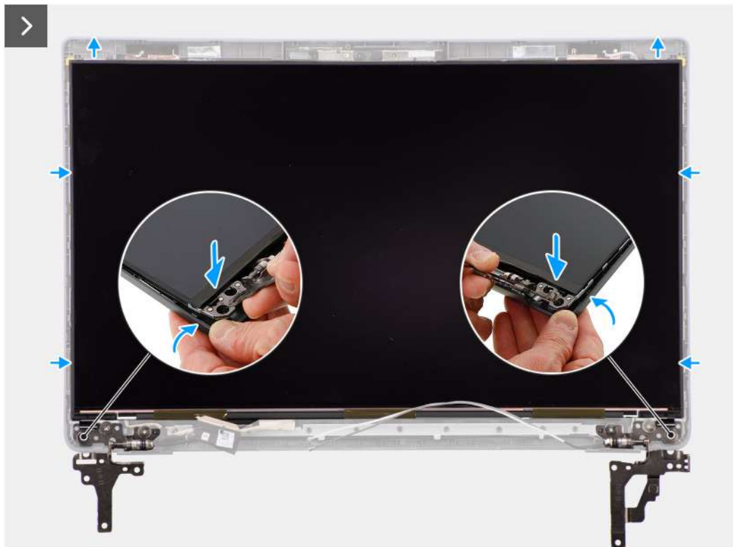
Figure 64. Installing the display panel
