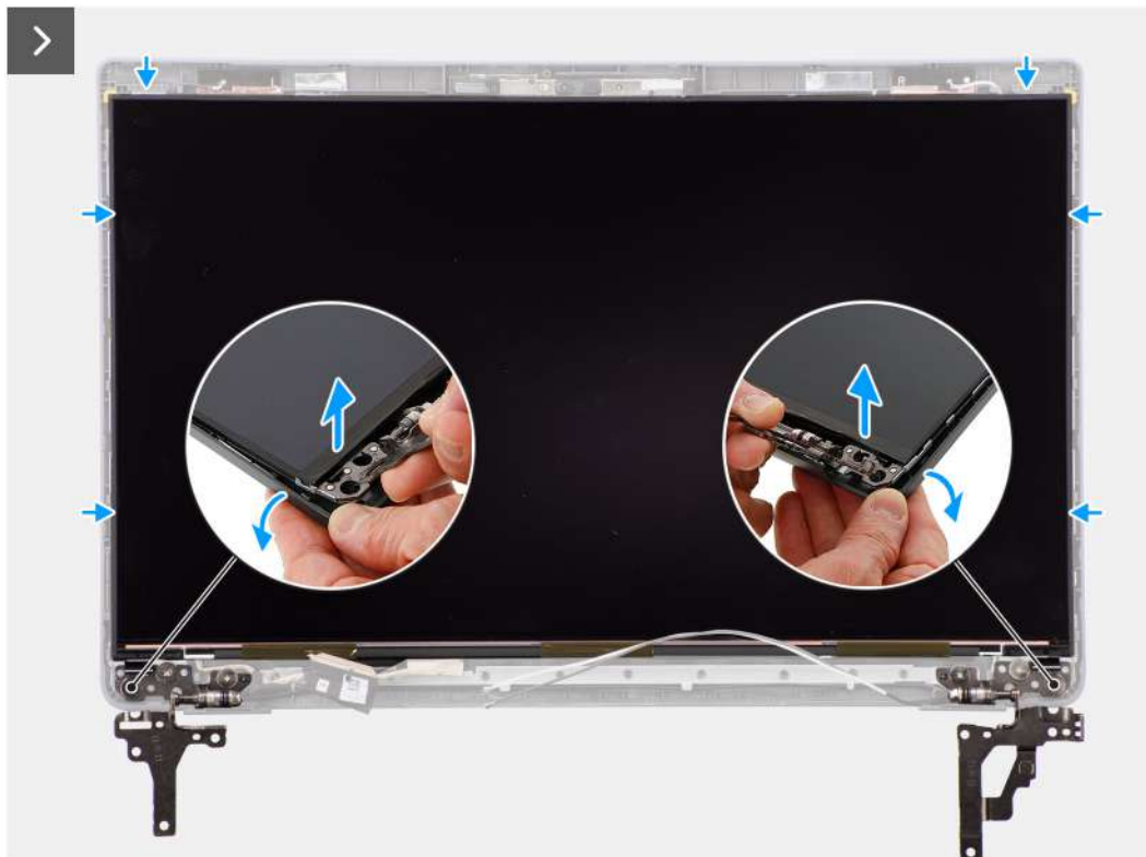
Figure 57. Removing the display panel
