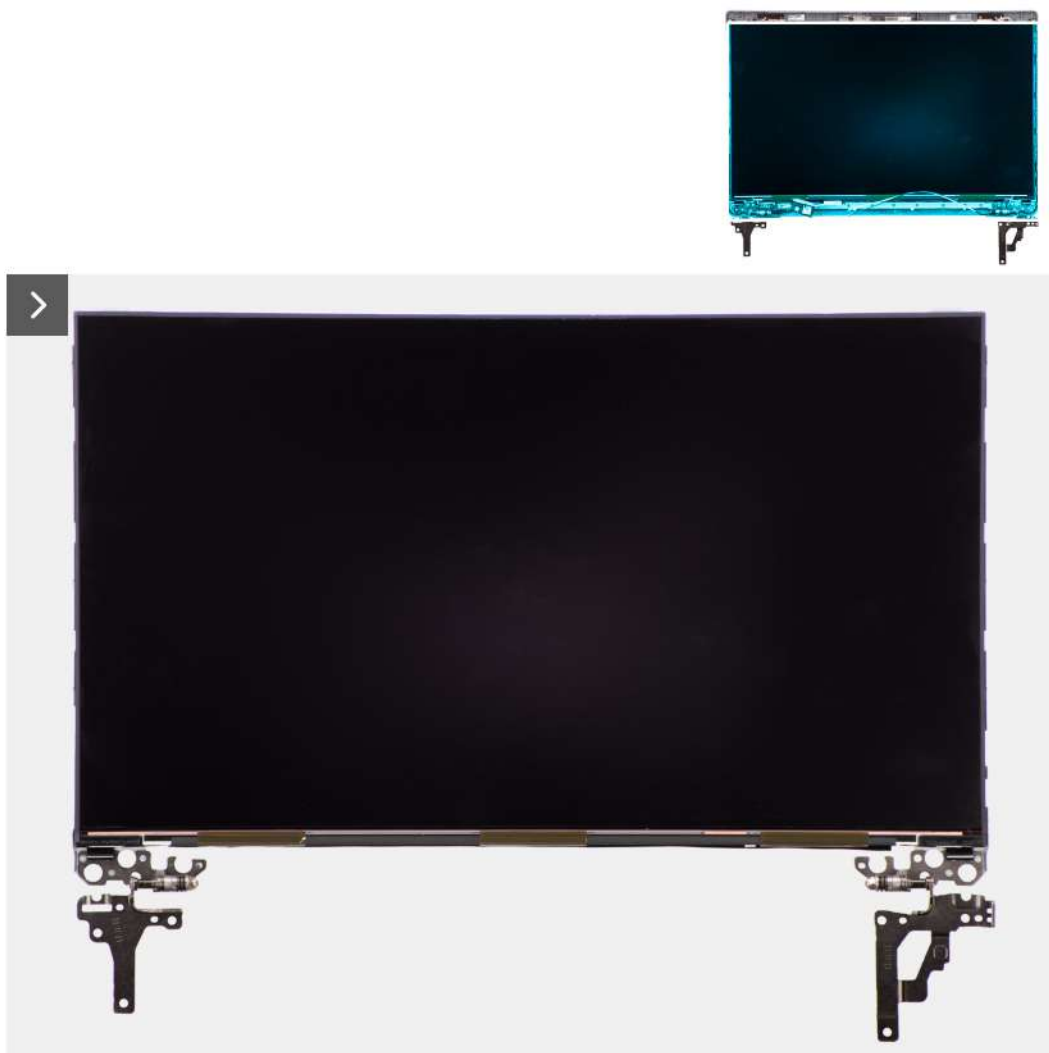
Figure 61. Installing the display panel
