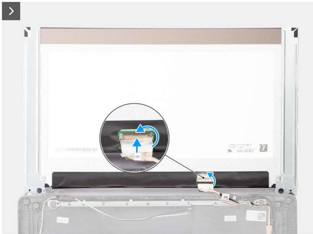
Figure 62. Installing the display panel
