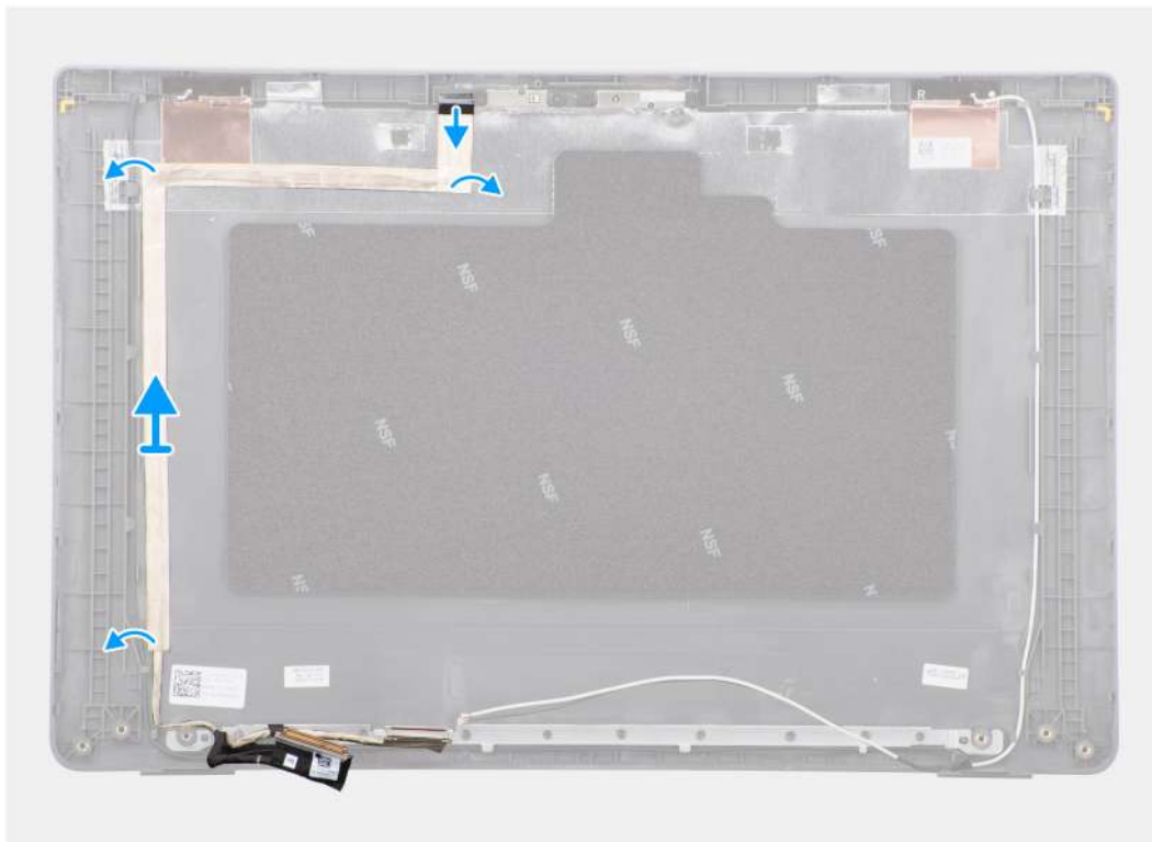
Figure 68. Removing the eDP cable
