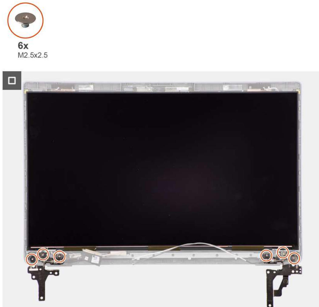
Figure 65. Installing the display panel
