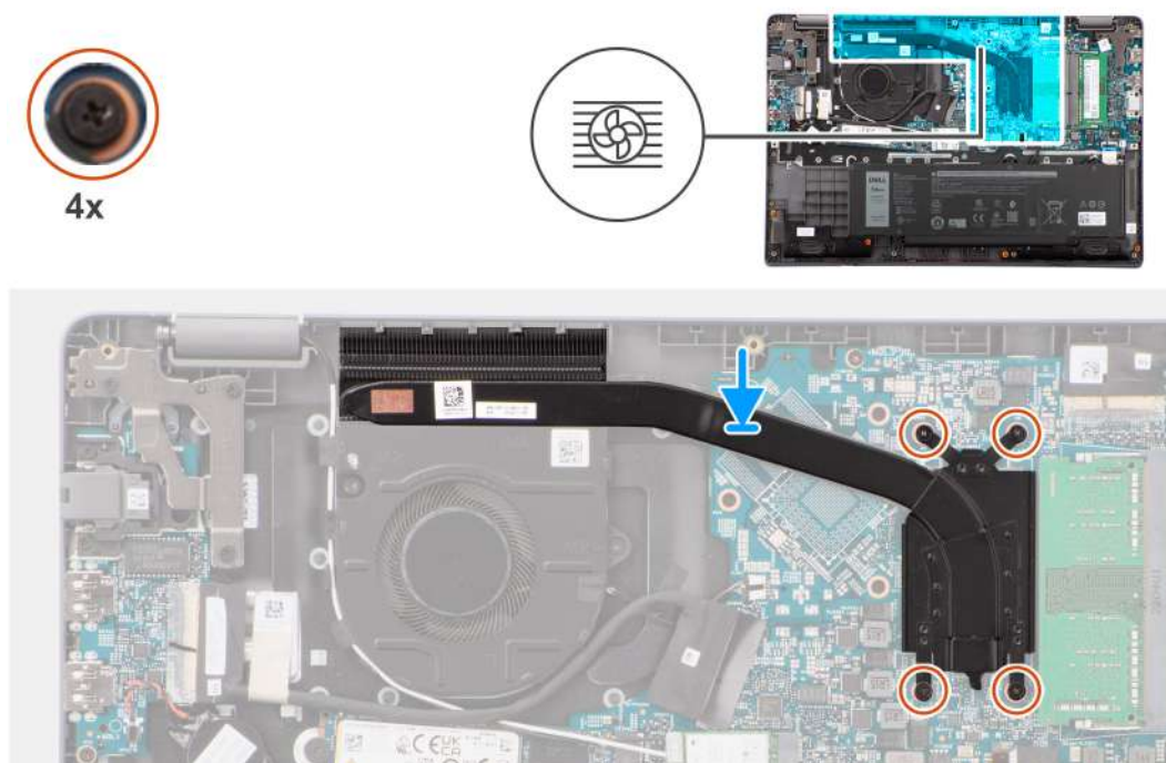
Figure 30. Installing the heat-sink for integrated graphics
