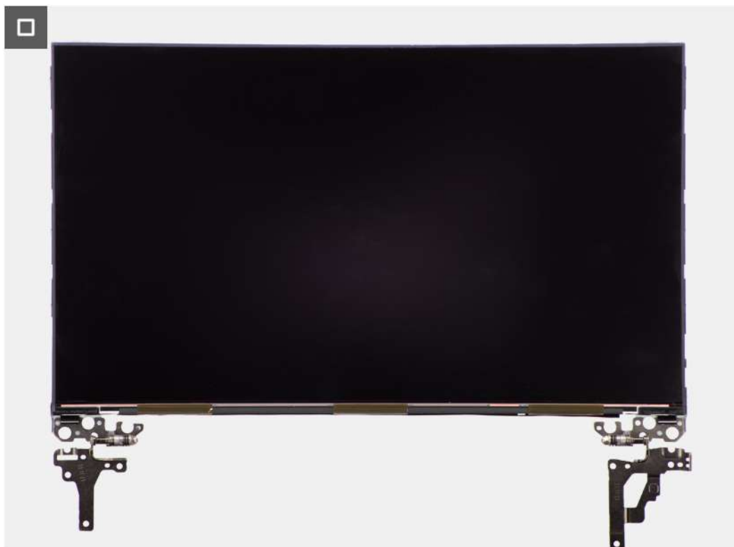
Figure 60. Removing the display panel
