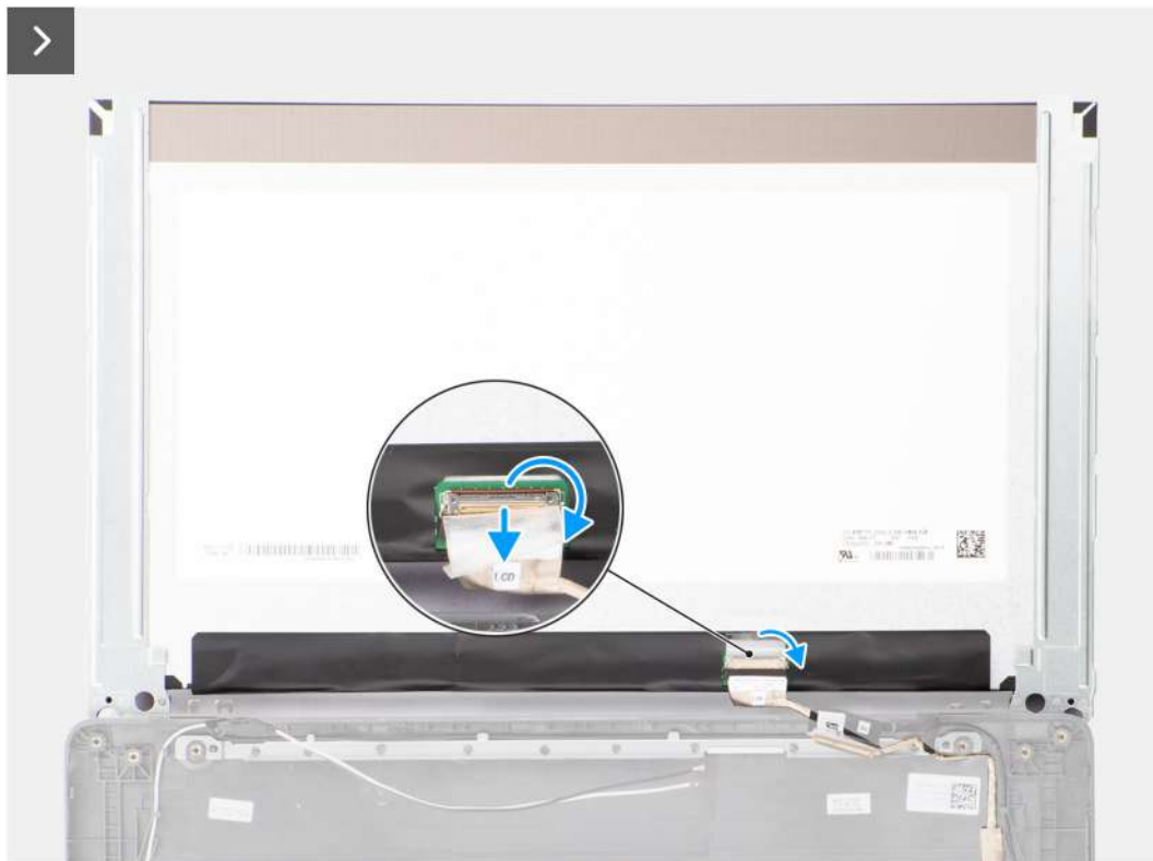
Figure 59. Removing the display panel
