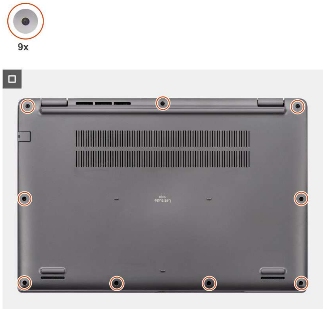
Figure 11. Installing the base cover
