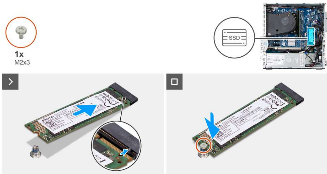
Figure 25. Installing the M.2 2280 solid state drive
