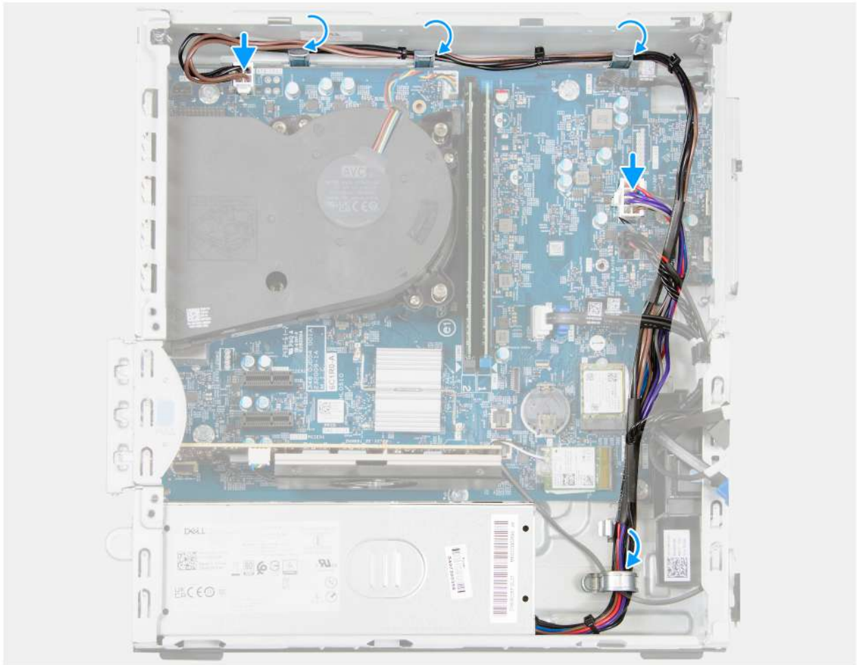
Figure 50. Installing the power-supply unit
