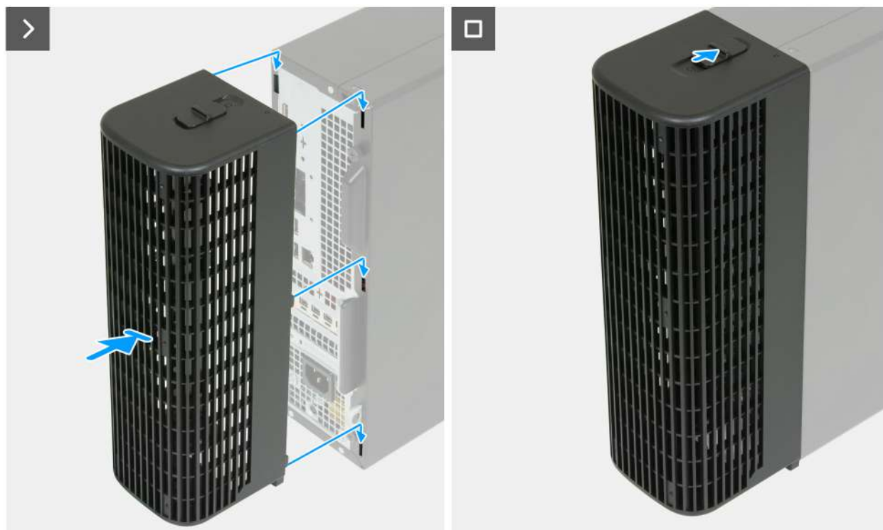
Figure 5. Installing the cable cover
