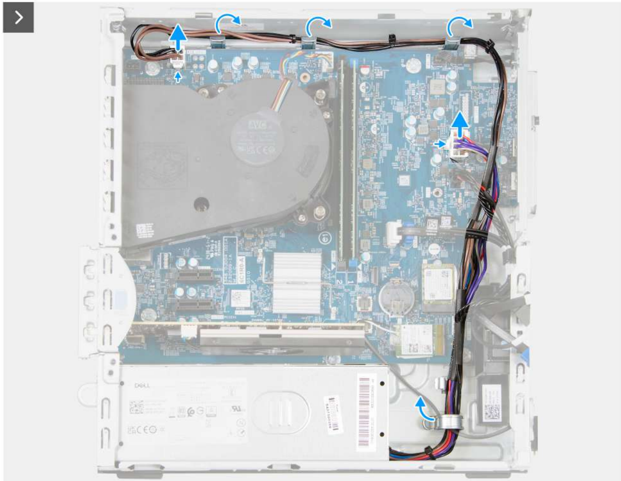
Figure 47. Removing the power-supply unit
