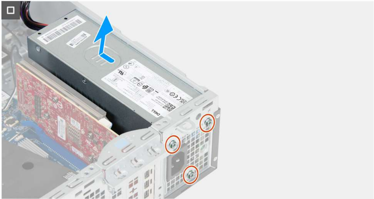
Figure 48. Removing the power-supply unit
