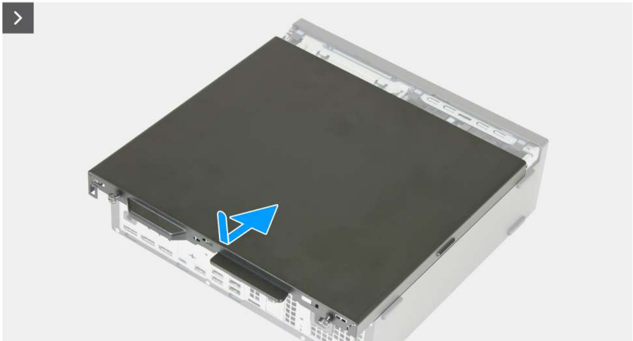
Figure 8. Installing the side cover
