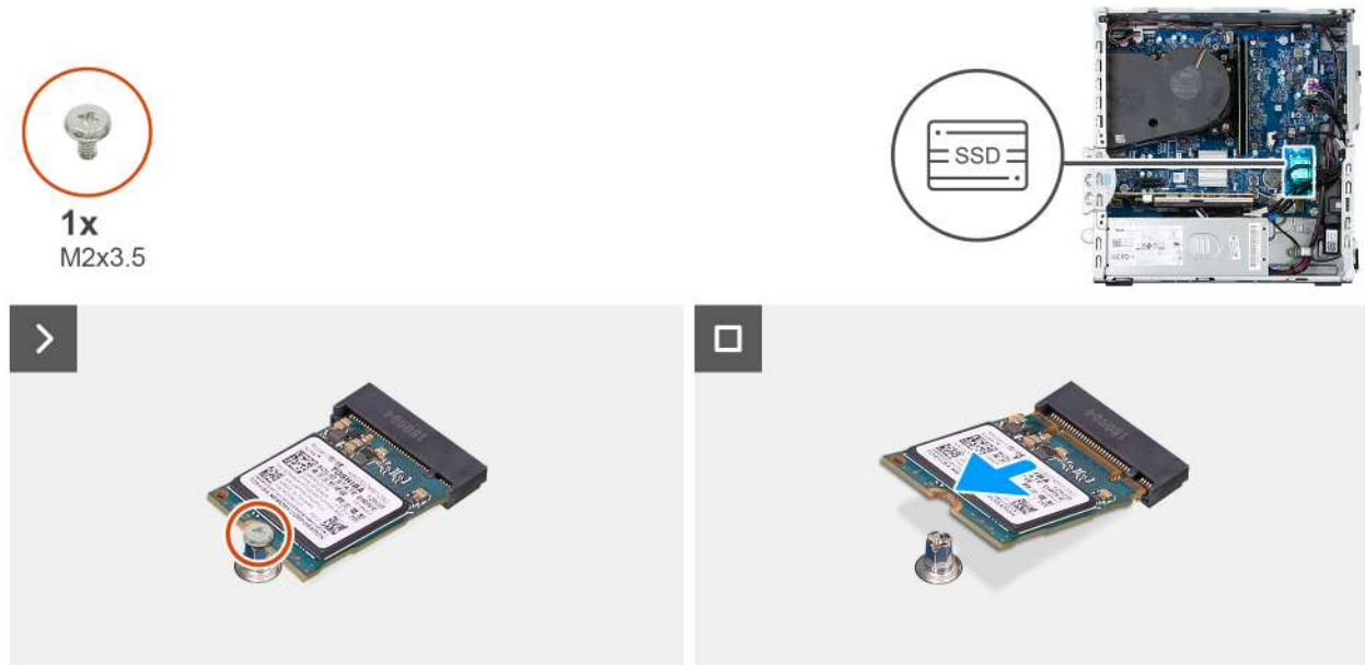
Figure 22. Removing the M.2 2230 solid state drive
