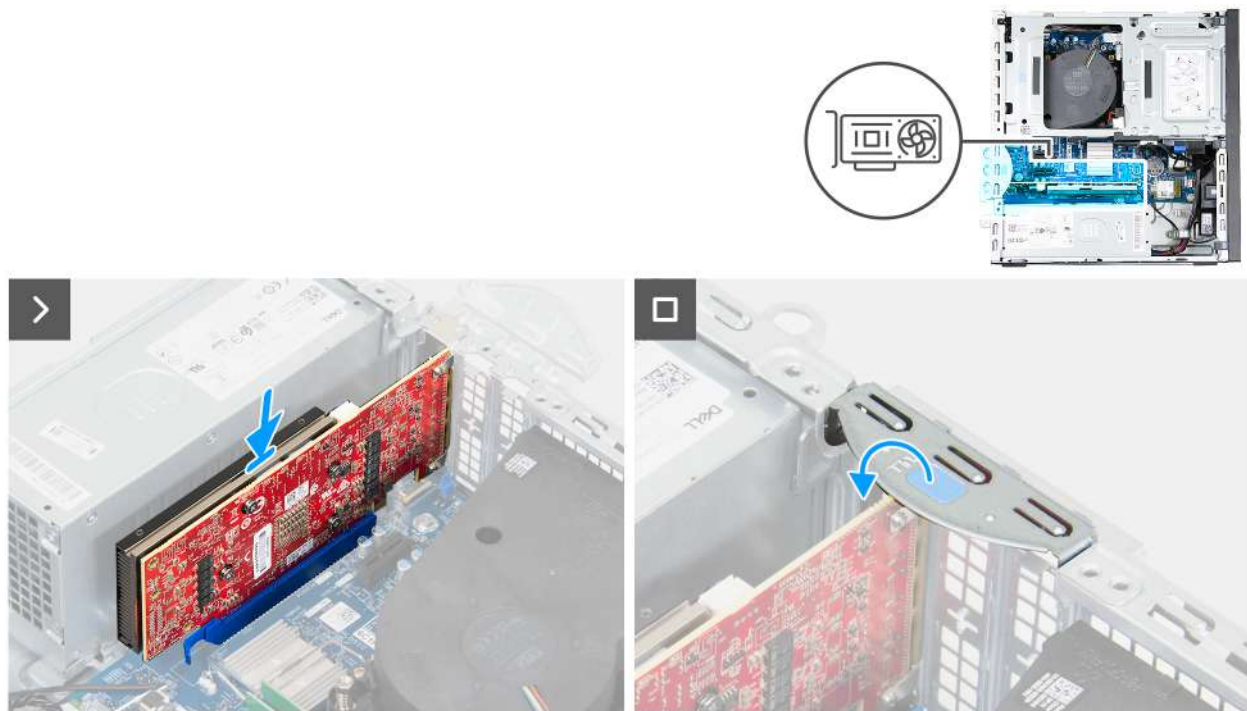
Figure 28. Installing the graphics card
