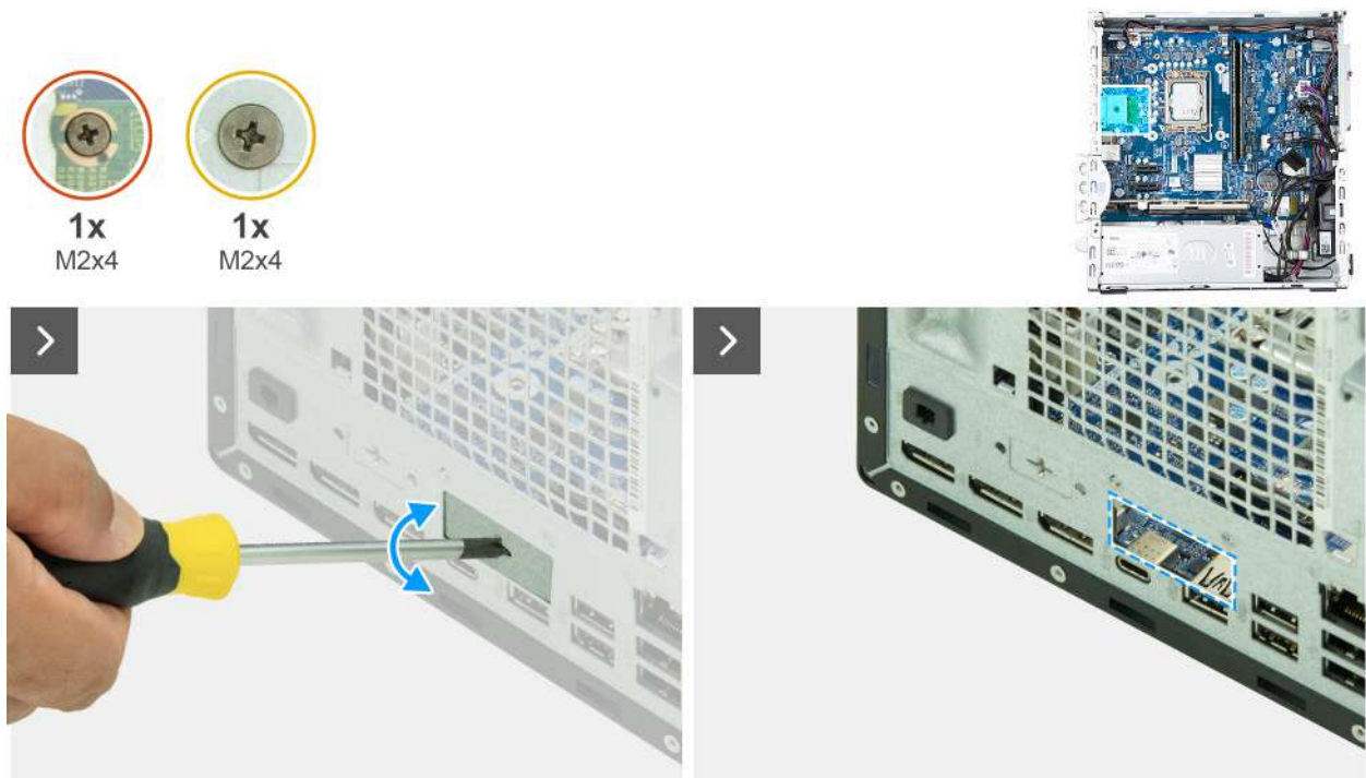
Figure 54. Installing the optional-port module
