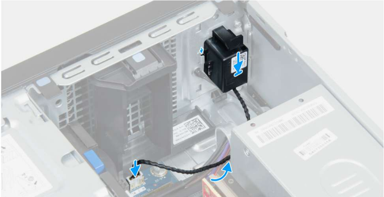
Figure 19. Installing the internal speaker
