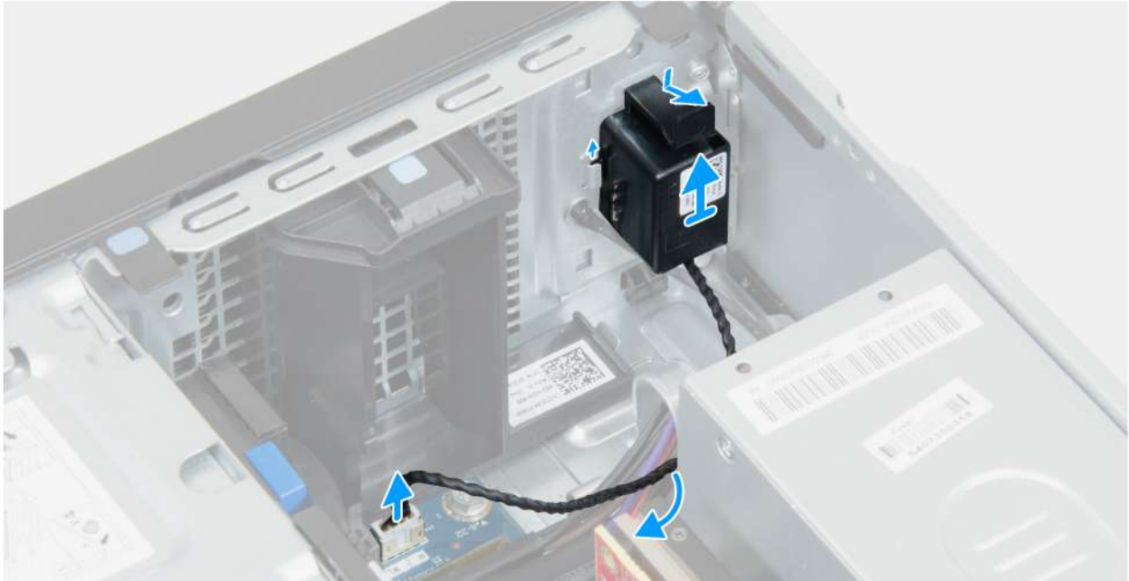
Figure 18. Removing the internal speaker
