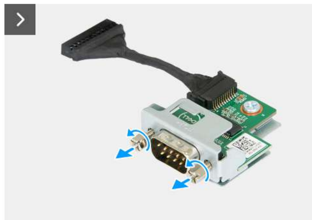
Figure 57. Installing the serial-port module
