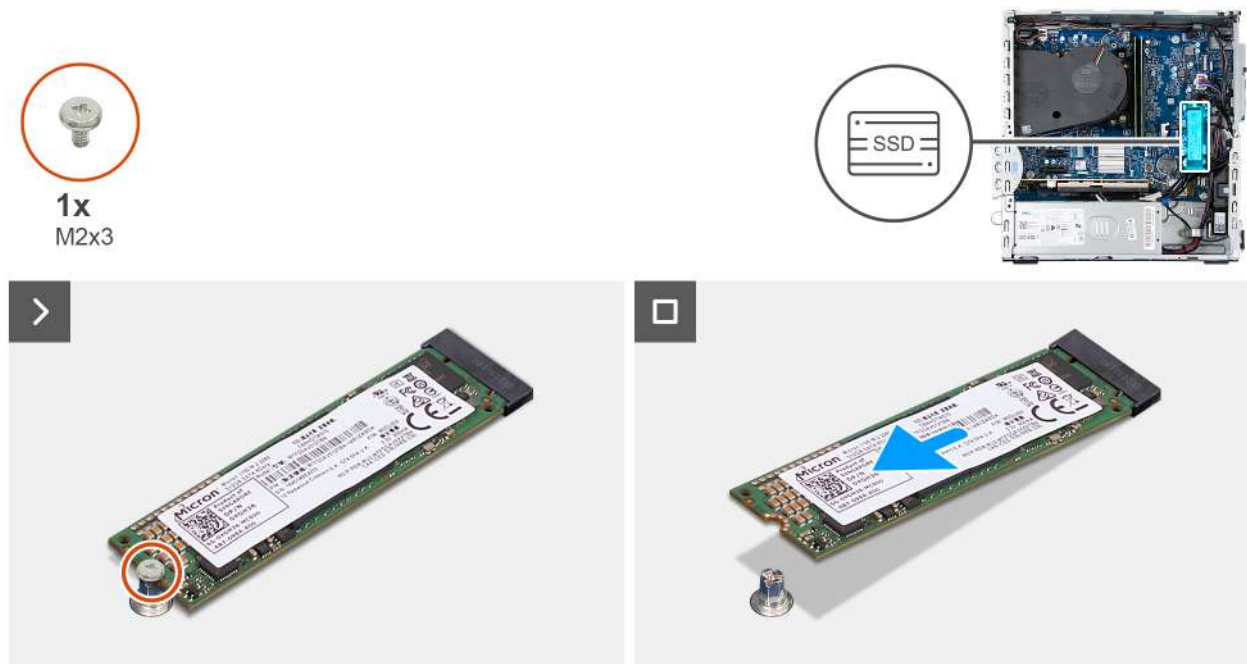
Figure 24. Removing the M.2 2280 solid state drive
