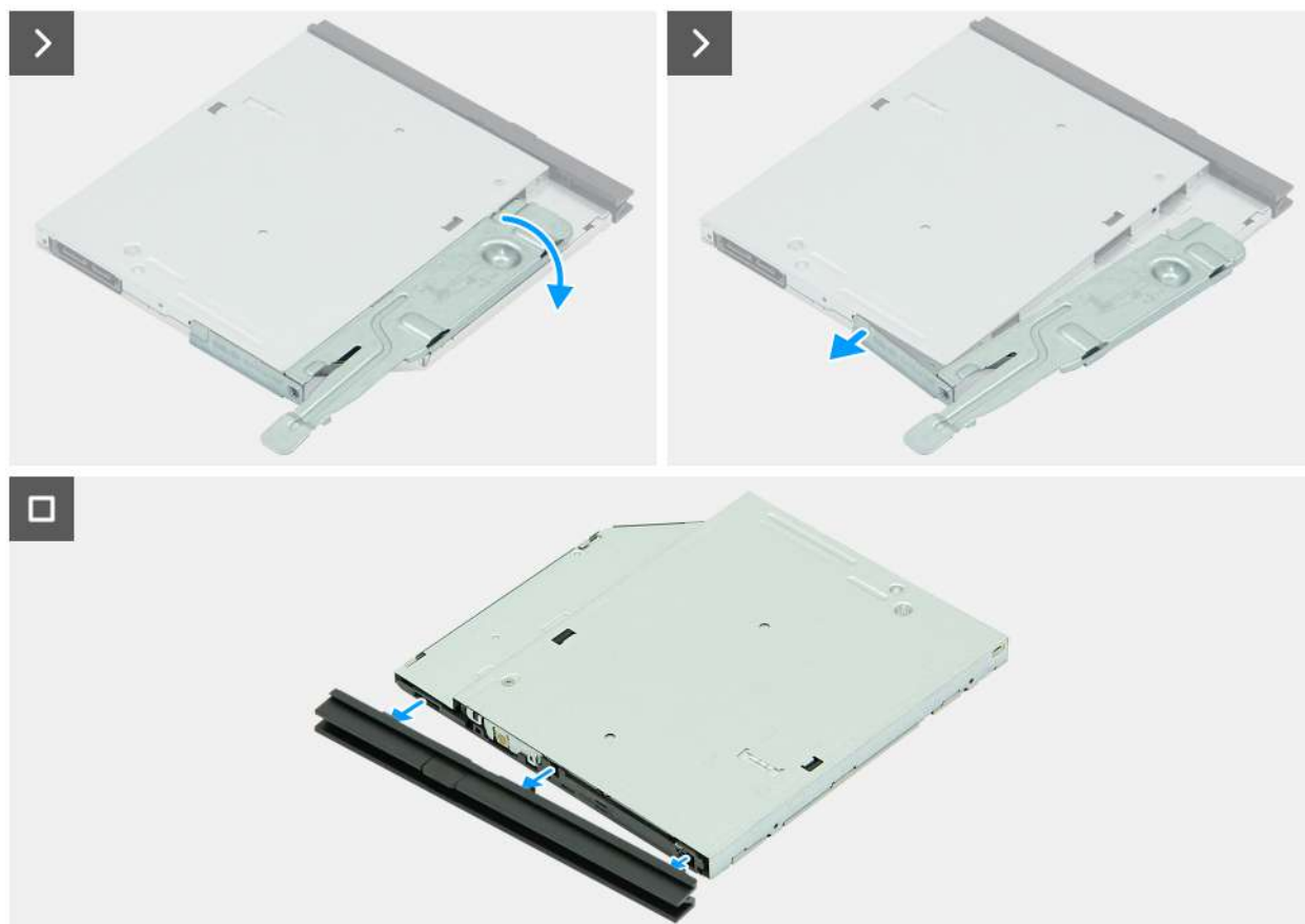
Figure 32. Removing the optical drive
