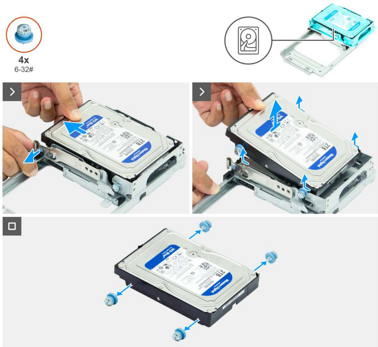
Figure 39. Removing the hard drive
