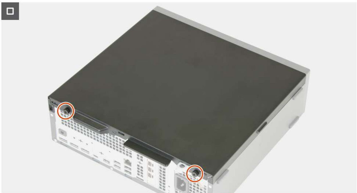
Figure 9. Installing the side cover
