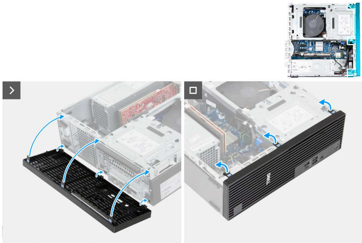
Figure 17. Installing the front cover
