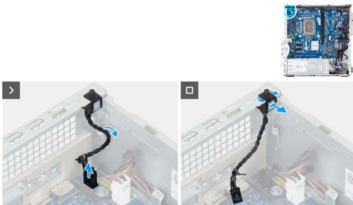
Figure 41. Removing the intrusion switch
