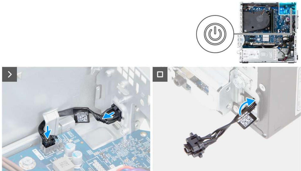
Figure 44. Installing the power button
