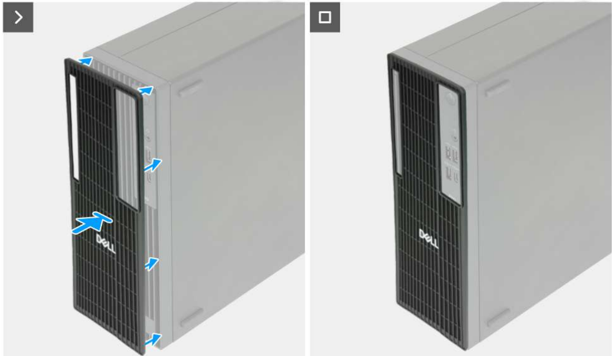
Figure 15. Installing the dust filter
