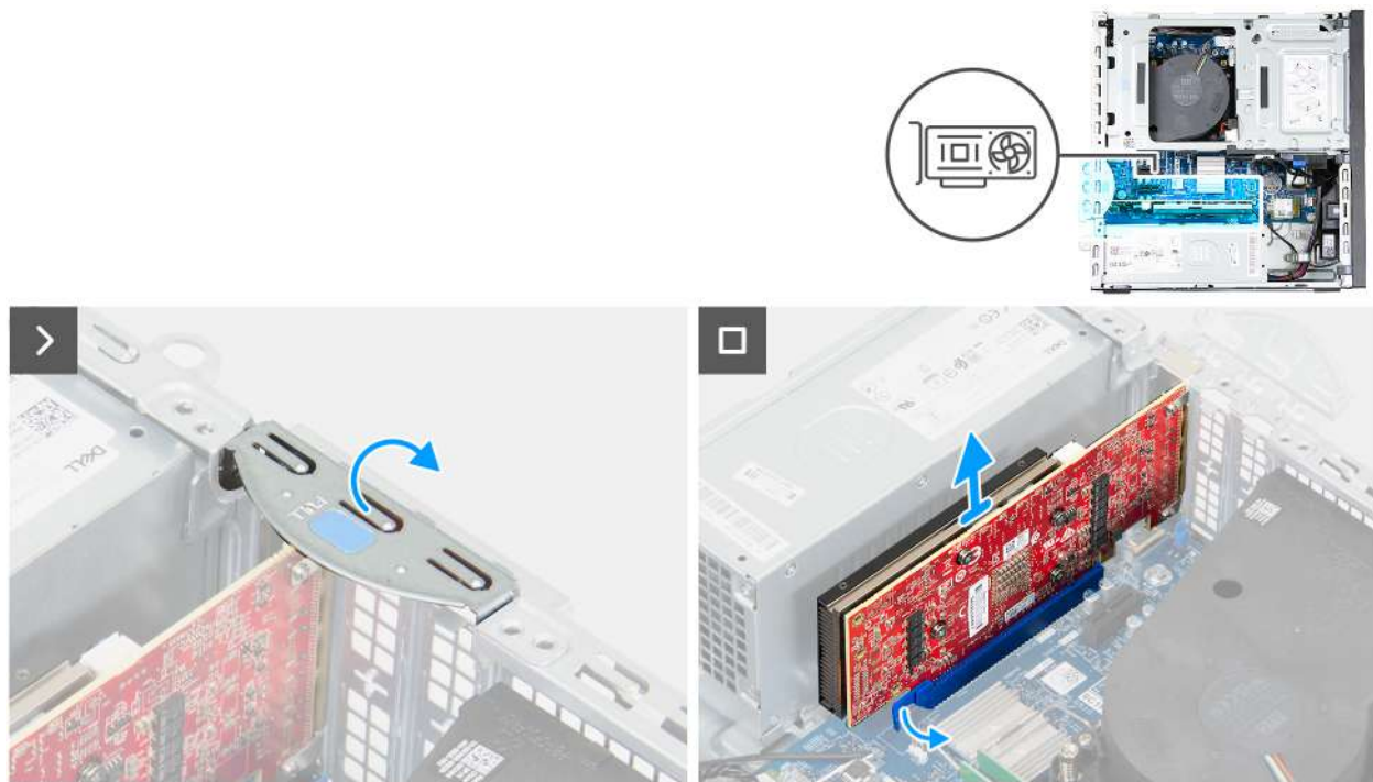
Figure 27. Removing the graphics card
