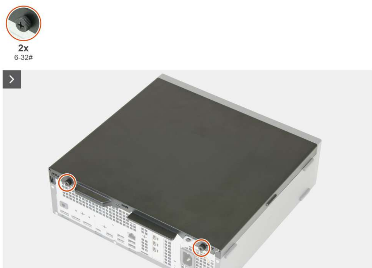
Figure 6. Removing the side cover
