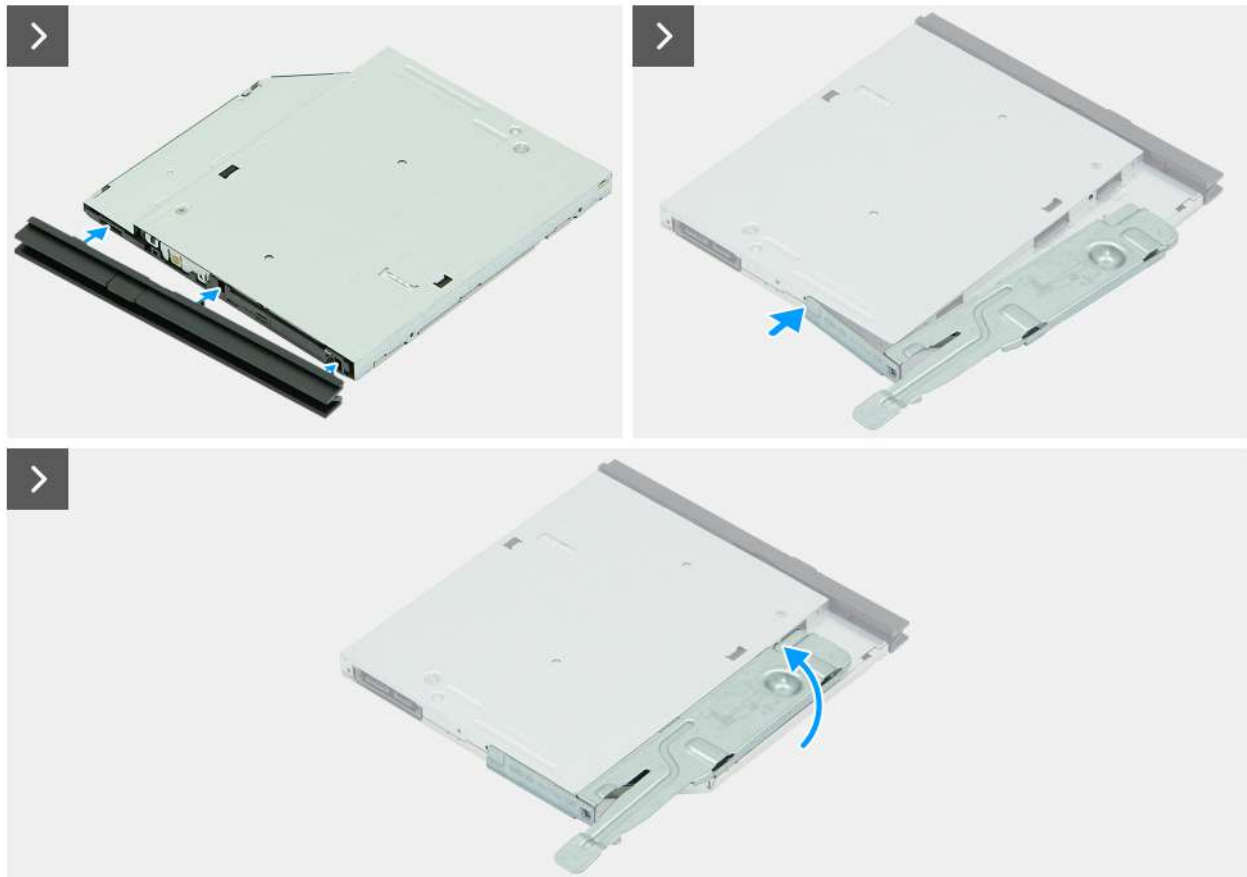
Figure 33. Installing the optical drive
