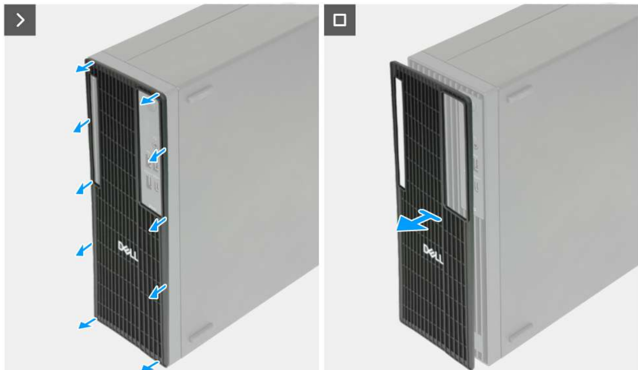
Figure 14. Removing the dust filter
