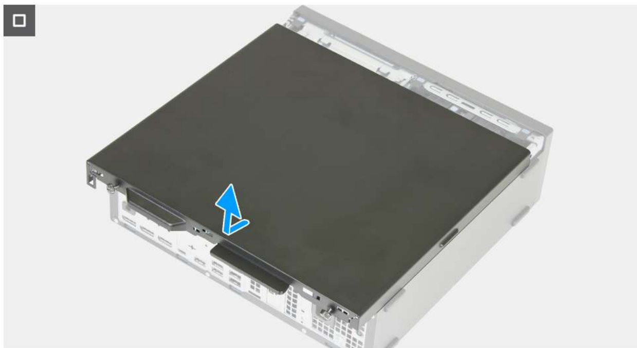
Figure 7. Removing the side cover
