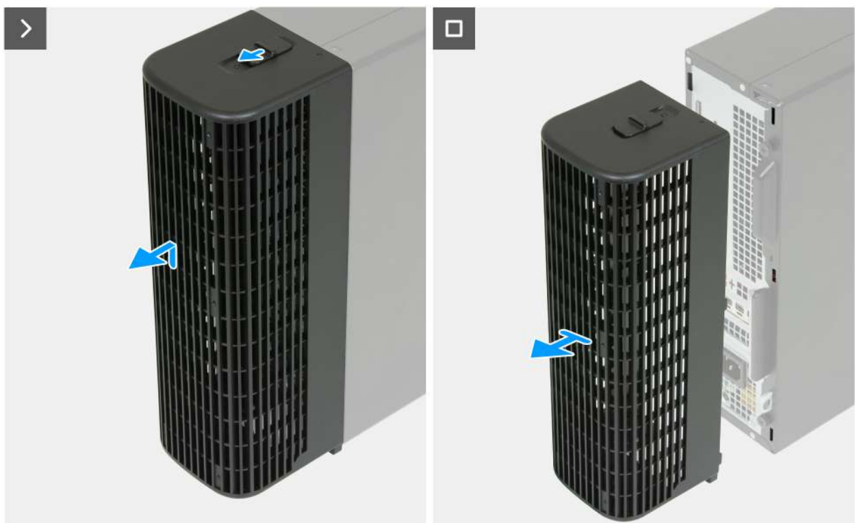
Figure 4. Removing the cable cover
