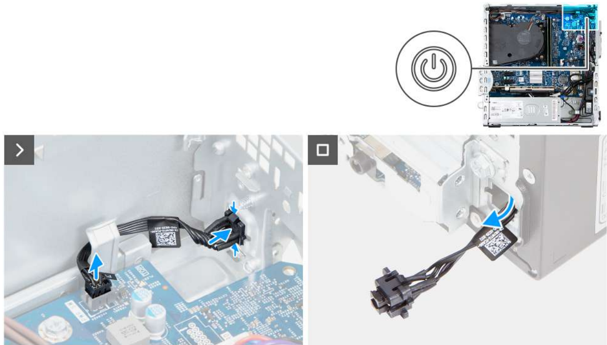
Figure 43. Removing the power button
