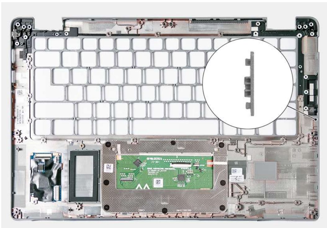
Figure 83. Removing the palm-rest assembly
