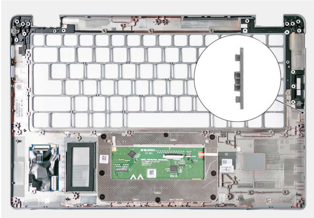
Figure 84. Installing the palm-rest assembly
