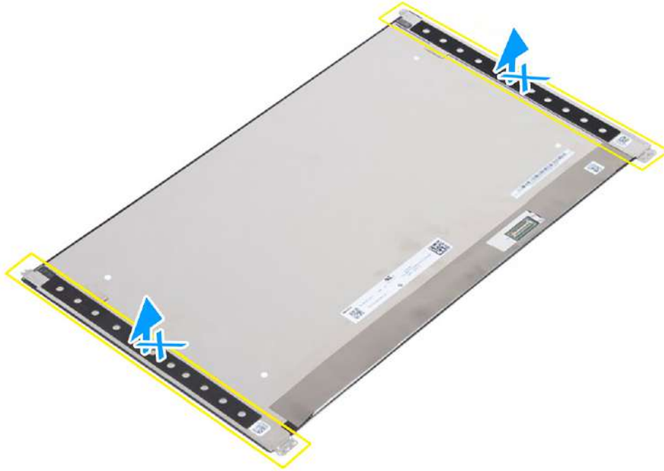
Figure 79. Do not pull and release the Stretch Release (SR) tapes
