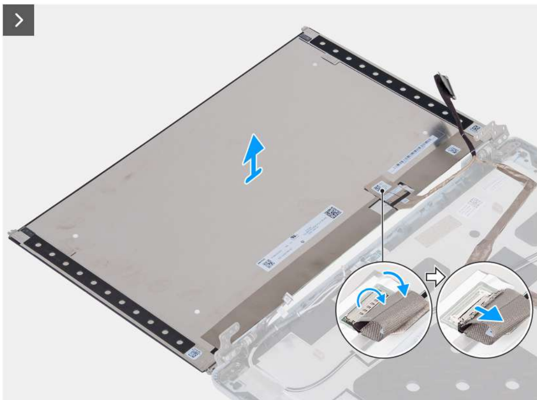
Figure 78. Removing the display panel
