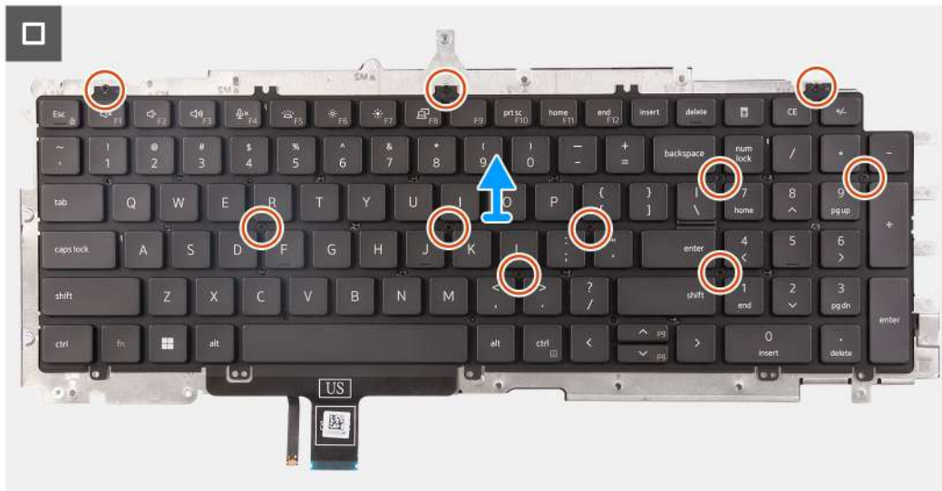
Figure 66. Removing the keyboard
