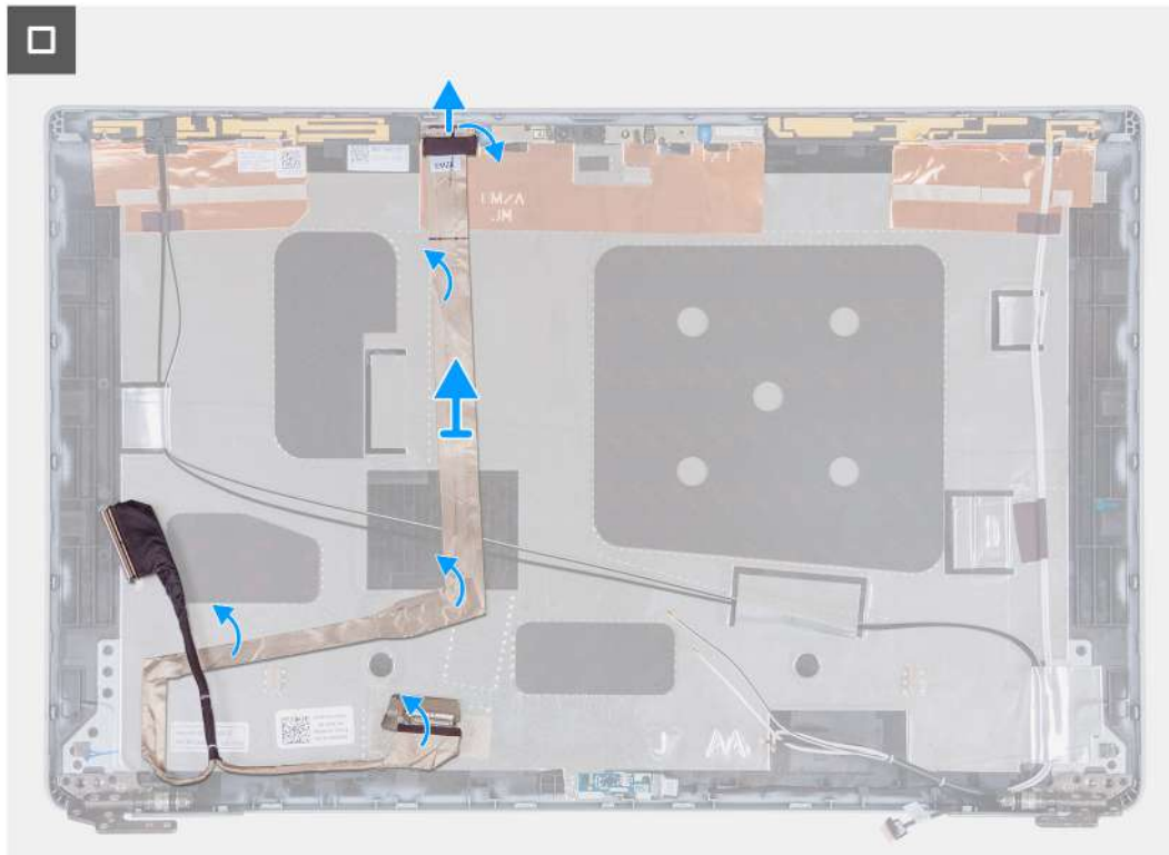
Figure 90. Removing the display cable
