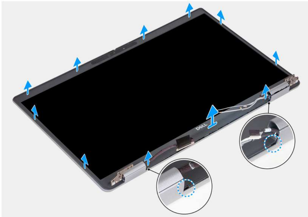
Figure 74. Removing the display bezel
