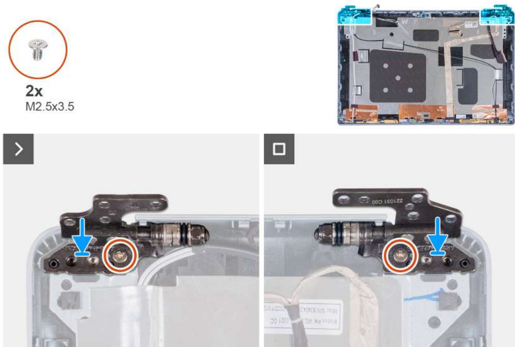
Figure 87. Installing the display hinges
