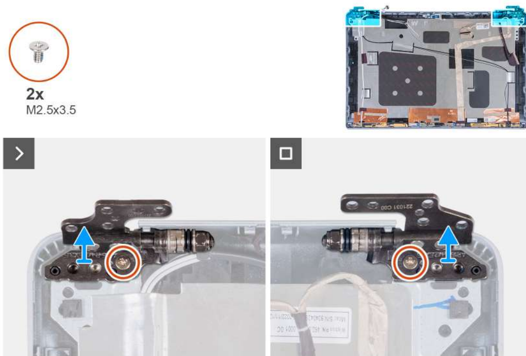
Figure 86. Removing the display hinges
