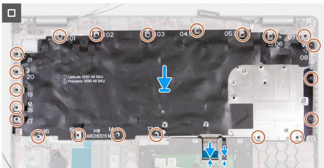
Figure 68. Installing the keyboard
