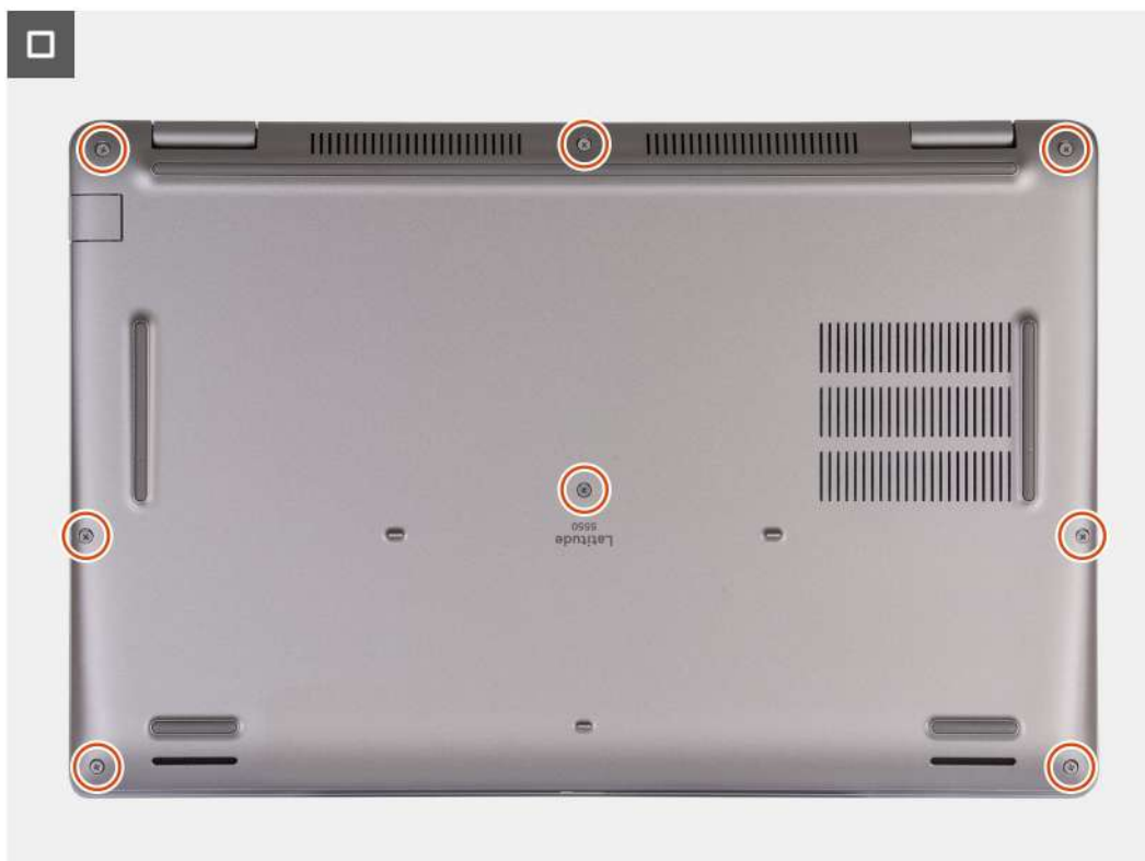
Figure 18. Tighten the captive screws
