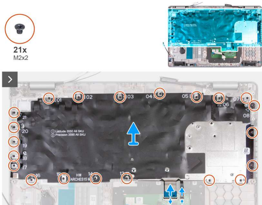
Figure 65. Removing the keyboard
