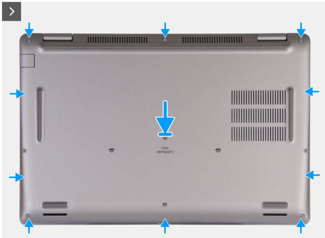
Figure 17. Installing the base cover
