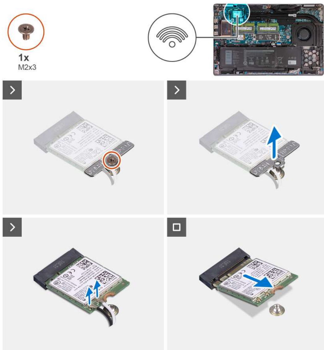
Figure 19. Removing the wireless card
