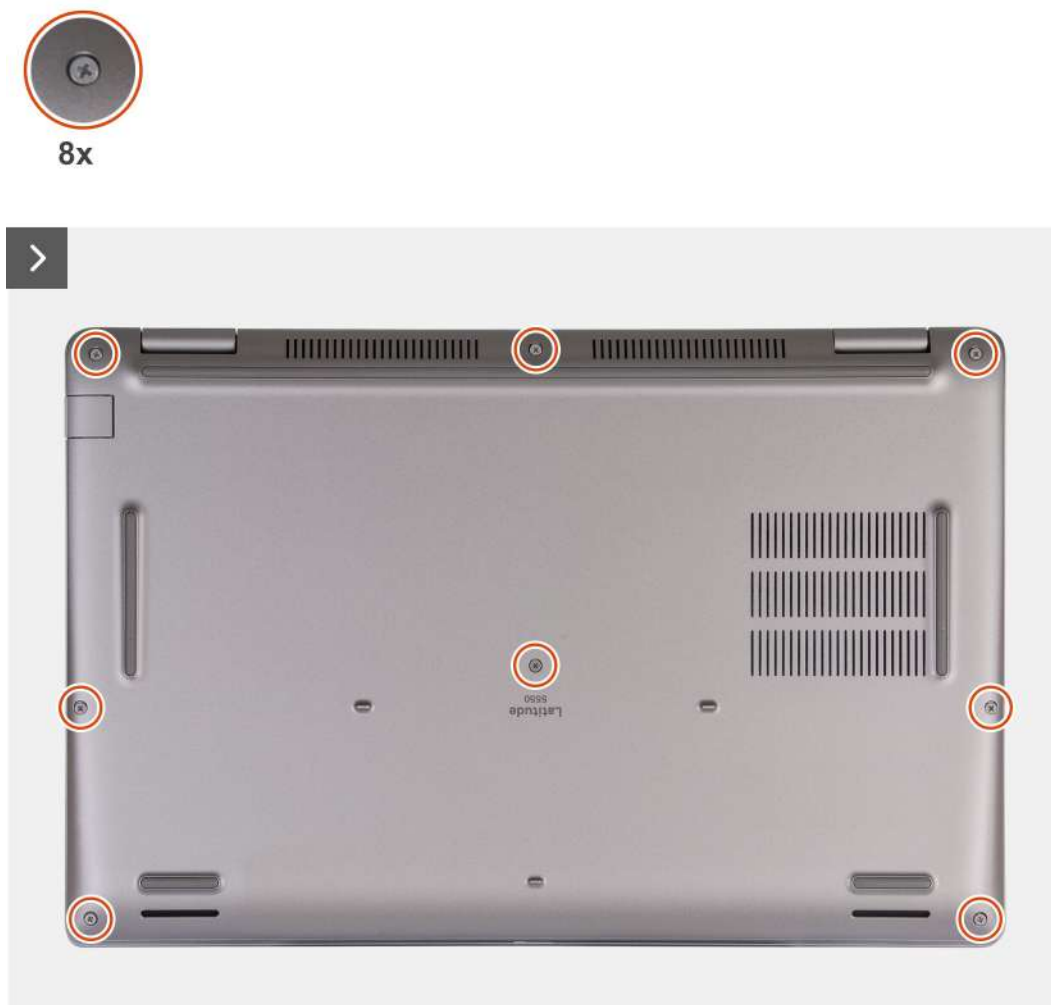
Figure 13. Loosen the captive screws
