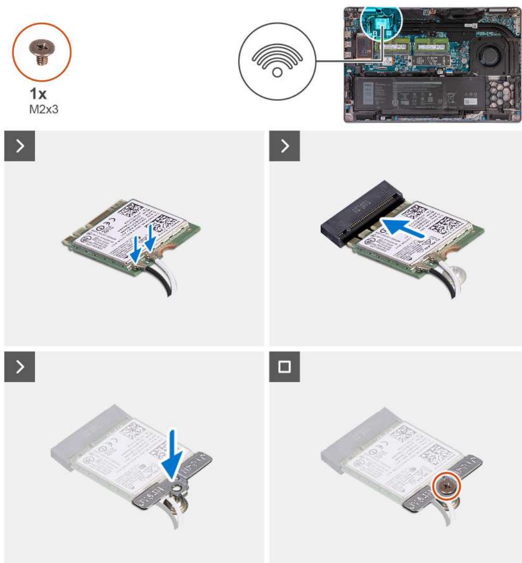
Figure 20. Installing the wireless card
