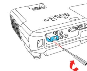
**Note:** The light on the wireless LAN module turns on when the module is installed and operating. The light flashes when the module is communicating over the network.
